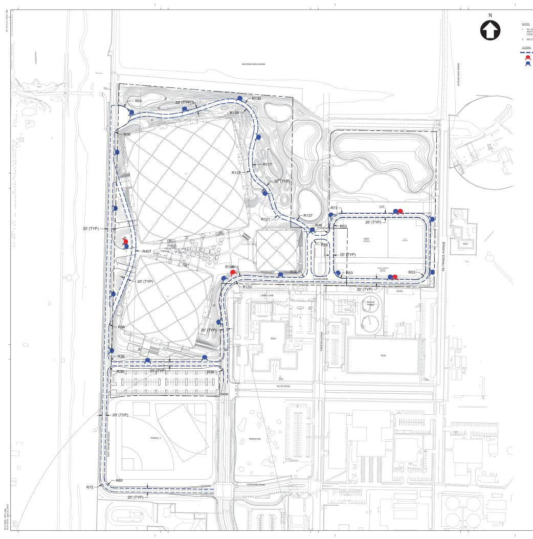
ALL ACCESS ROADS WILL HAVE A TYPICAL WIDTH OF 20' AND AN INCREASED WIDTH OF 26' NEAR FIRE HYDRANTS IN ACCORDANCE WITH THE CALIFORNIA FIRE CODE 2013 (OR MOST RECENT VERSION) SECTION D103.1. 2. SEE DETAIL 1 FOR MINIMUM CLEARANCE AROUND A FIRE HYDRANT
