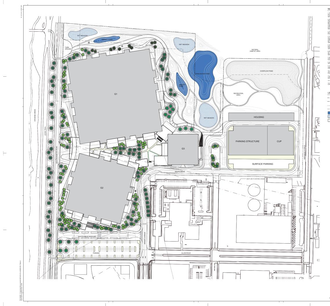
1. ALL AREAS NOT COVERED BY BUILDINGS OR PAVEMENT AND WHICH HAVE BEEN GRADED OR OTHERWISE DISTURBED SHALL BE TOPSOILED AND SEEDED, UNLESS SHOWN OTHERWISE.
