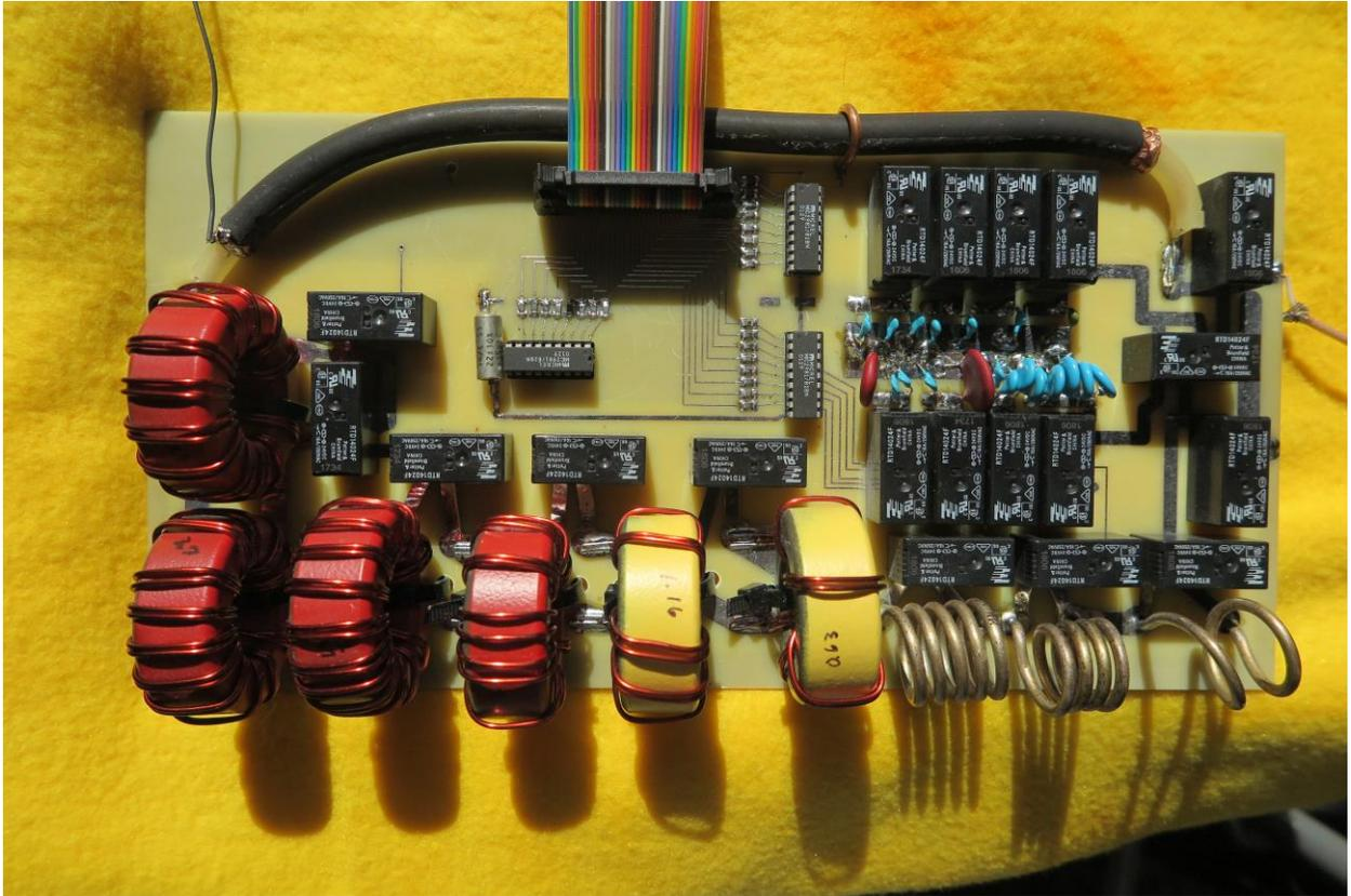
The integrated circuits are relay drivers with 24 VDC as the supply, and standard TTL levels which come in through the ribbon cable as switching lines. The TTL lines are low-pass filtered to try and keep the healthy amounts of RF floating around on the board from affecting the switching circuits.
